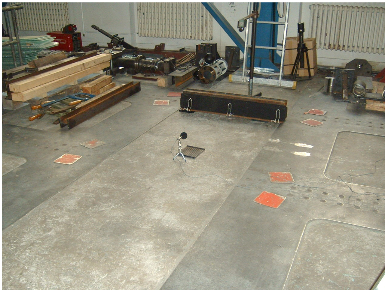
Fig. 1 View of the measurement location, absorber attached to the rail with clips
