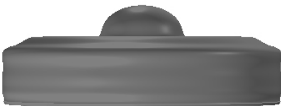
Fig. 1: Illustration of the traditional gamelan gong (a) orthogonal views and the top-side plane perspectives, and (b) cross-sectional profile modeled in 2D axisymmetric coordinates.
