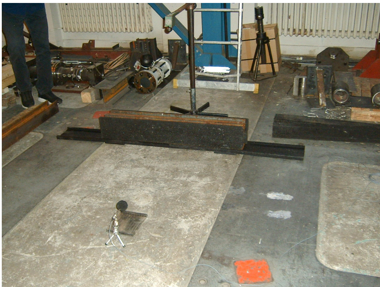
Fig. 2 View of the measurement location, absorber attached to the rail by gluing
