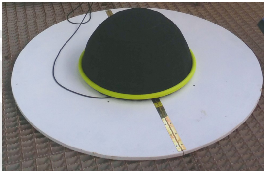
Fig.3: Dome used in the urban area according to IEC 61400-11[10]
