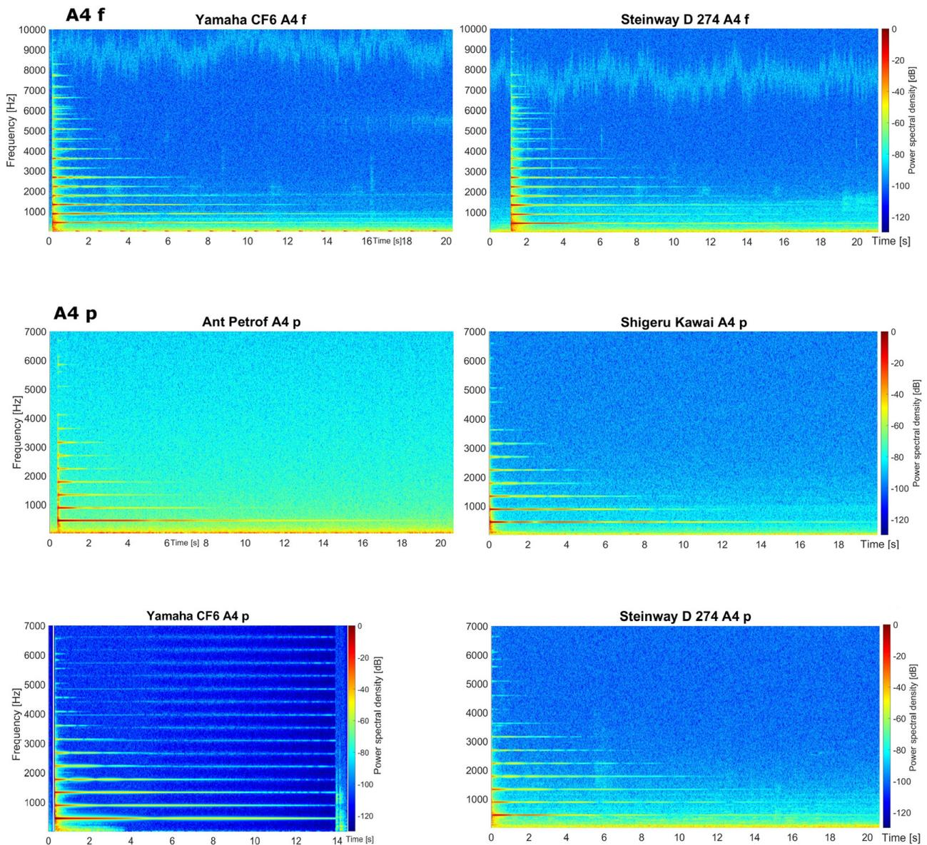
Figure 11. Comparison of tone A4 (one-line A) in dynamics *f* and *p*
