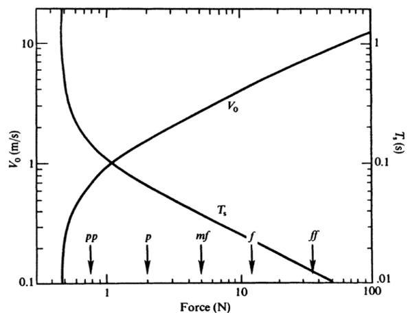
Figure 2. Hammer velocity ( $V_0$ ) and key depressing time ( $T_s$ ) for different values of force (assumed to be constant during the time  $T_s$ ) [2]
