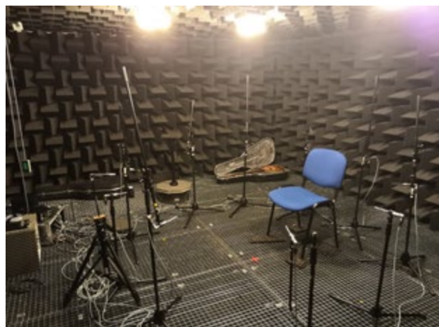
Fig. 4: Measurement of spectra and sound radiation in the anechoic room of Brno University of Technology
