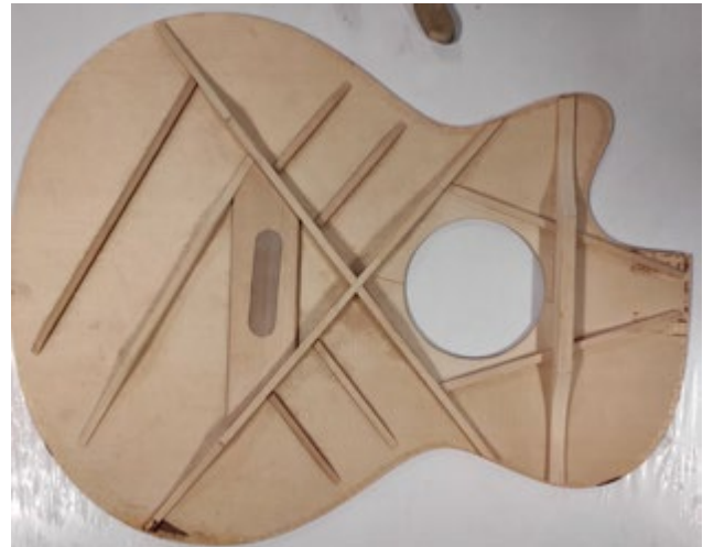
Fig 2: Dreadnought top plate braces
